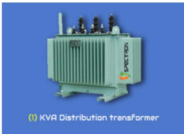
In general, Distribution Transformer is used to reduce primary system voltages (2.4-34.5KV) to utilization voltages (120-600) They are all power Transformers in the sense that their purpose is to transmit power from one voltage level to another,
